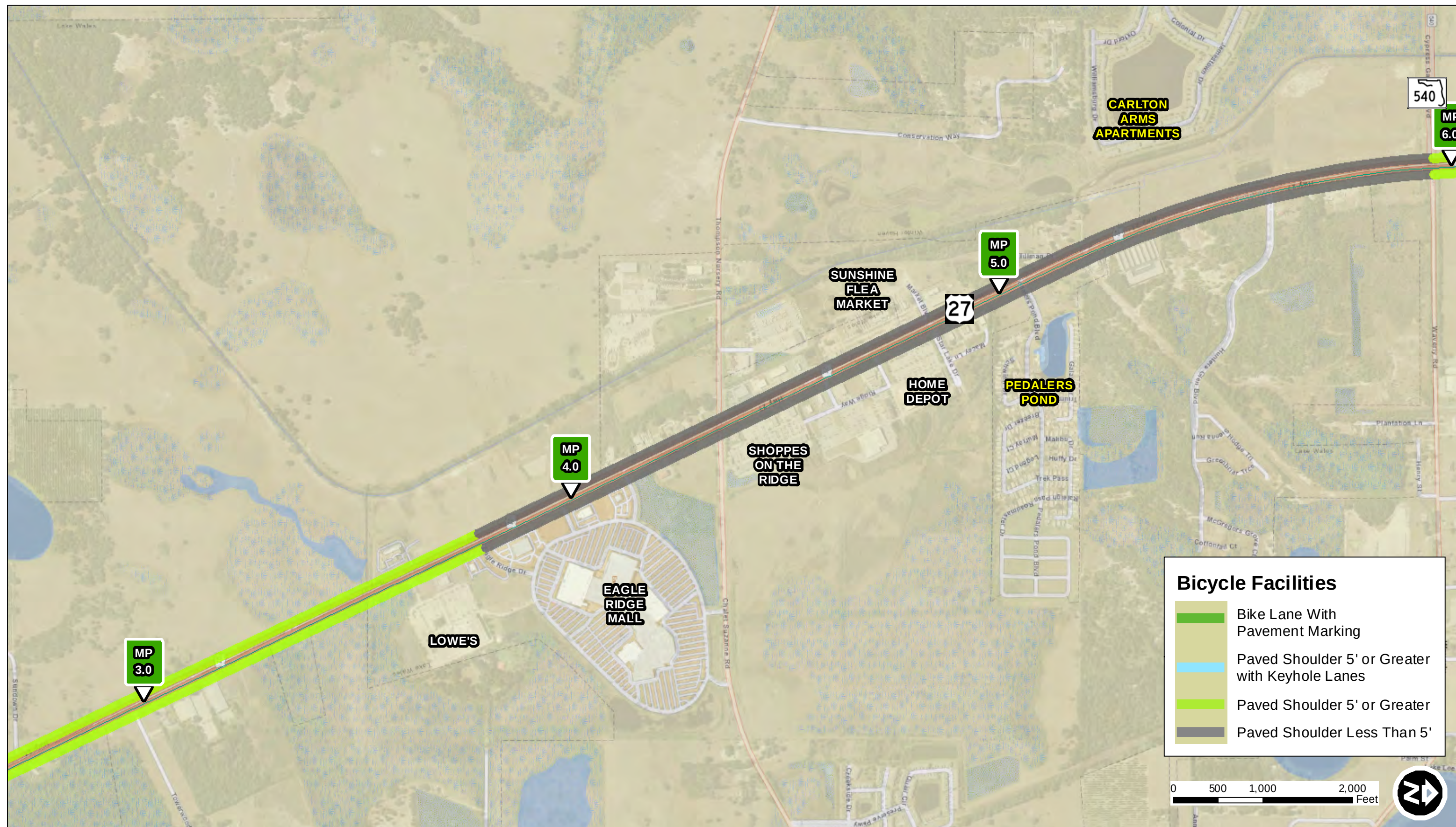
FIGURE 3-2 BICYCLE FACILITIES US 27 CORRIDOR Sheet 2 of 11
