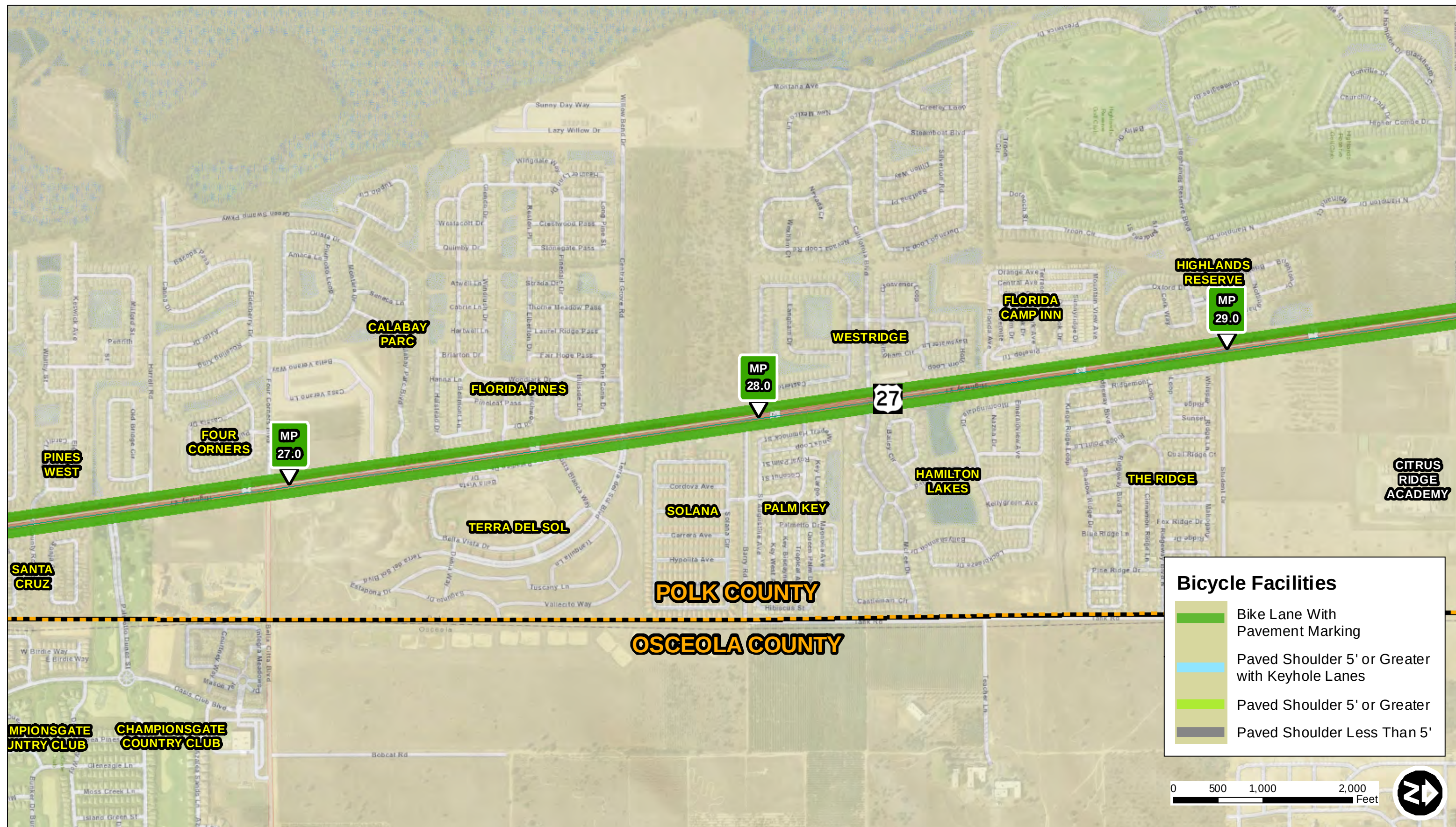
FIGURE 3-2 BICYCLE FACILITIES US 27 CORRIDOR Sheet 10 of 11
